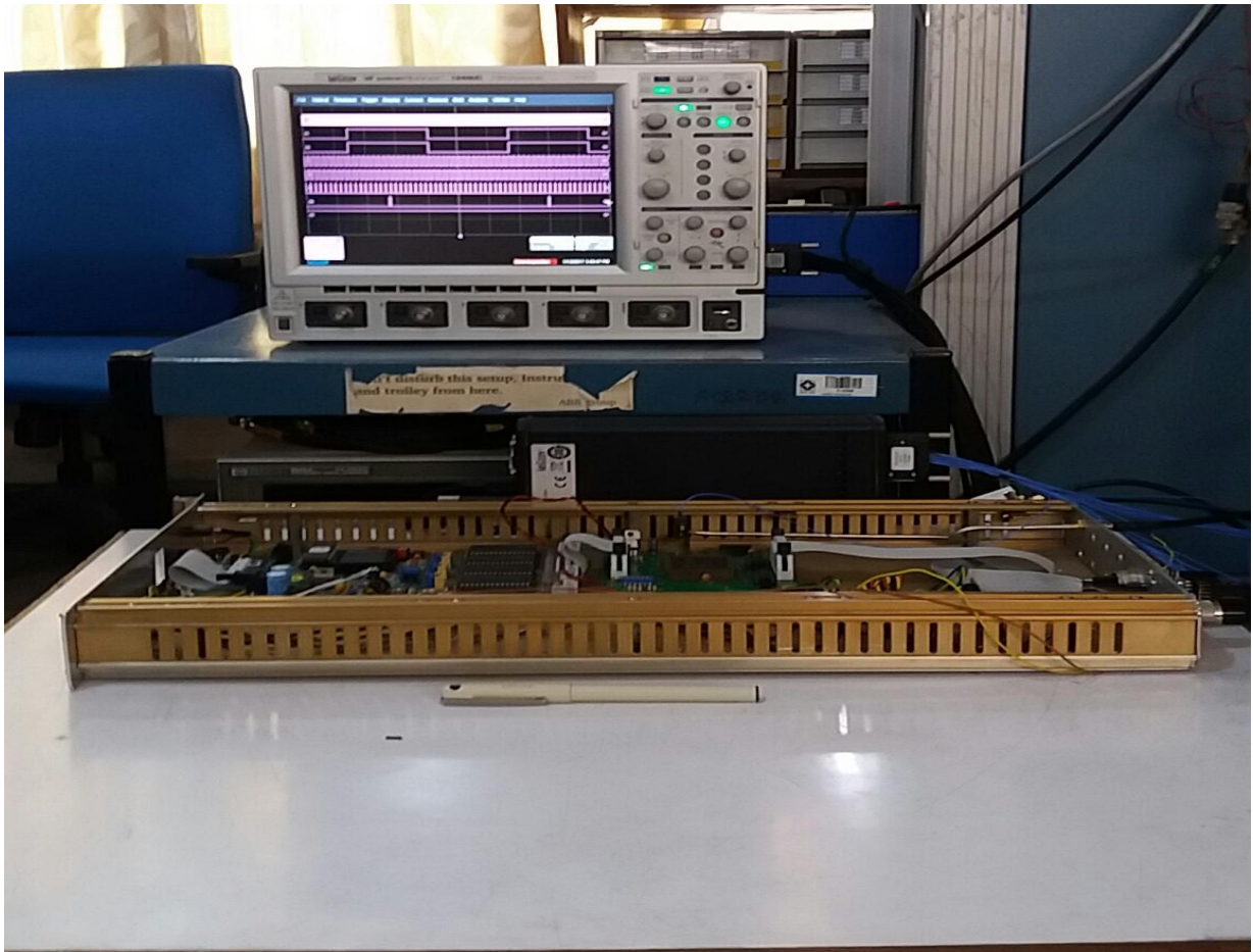
Figure 7: Snapshot of CPLD based FE and Walsh PIU lab test setup
